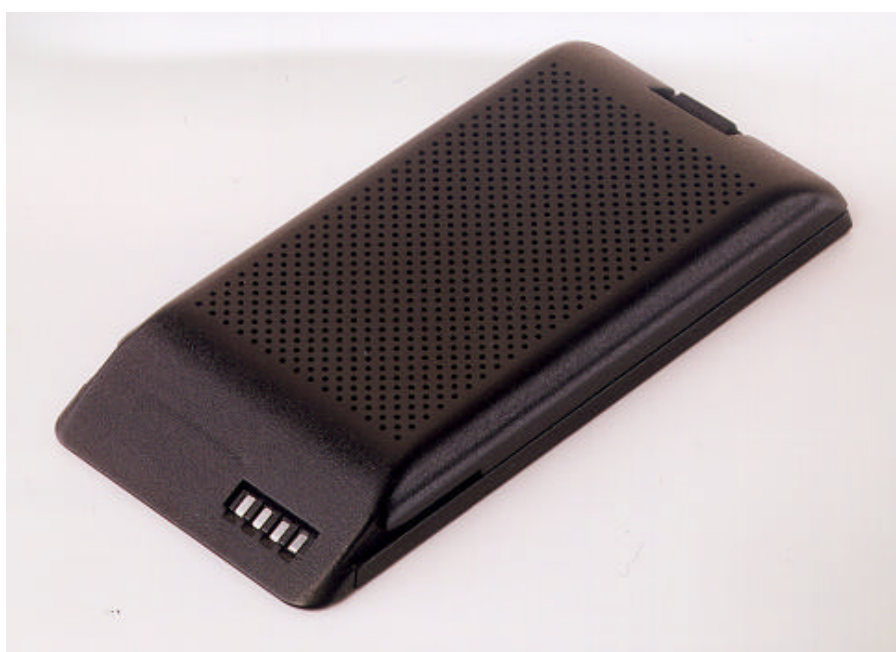
Fig. 8: 6 V Motorola battery with air holes in the pack wall to allow air access to the zinc-air cells within
